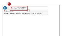
Open IE Browser and input IP Address of 727CM (Default IP address is http://192.168.1.127)
